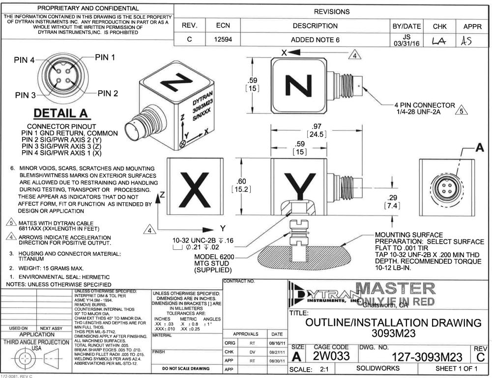
3093M23 PERFORMANCE SPECIFICATION DOC NO PS3093M23 Accelerometer, Triaxial, IEPE REV C, ECN 10287, 08/16/2013
