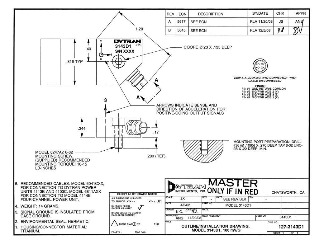
Model Number DOC NO PERFORMANCE SPECIFICATIONS 3143D1 PS3143D1 IEPE TRIAXIAL ACCELEROMETER REV A, ECN 11933 , 06/10/15
