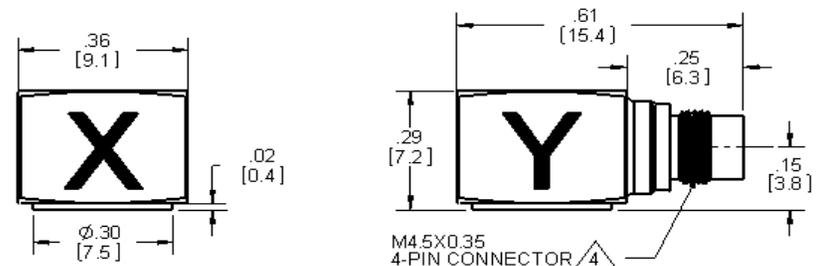
Units on the line drawing are in inches, units in brackets are in millimeters. Refer to 127-3343A for more information.
