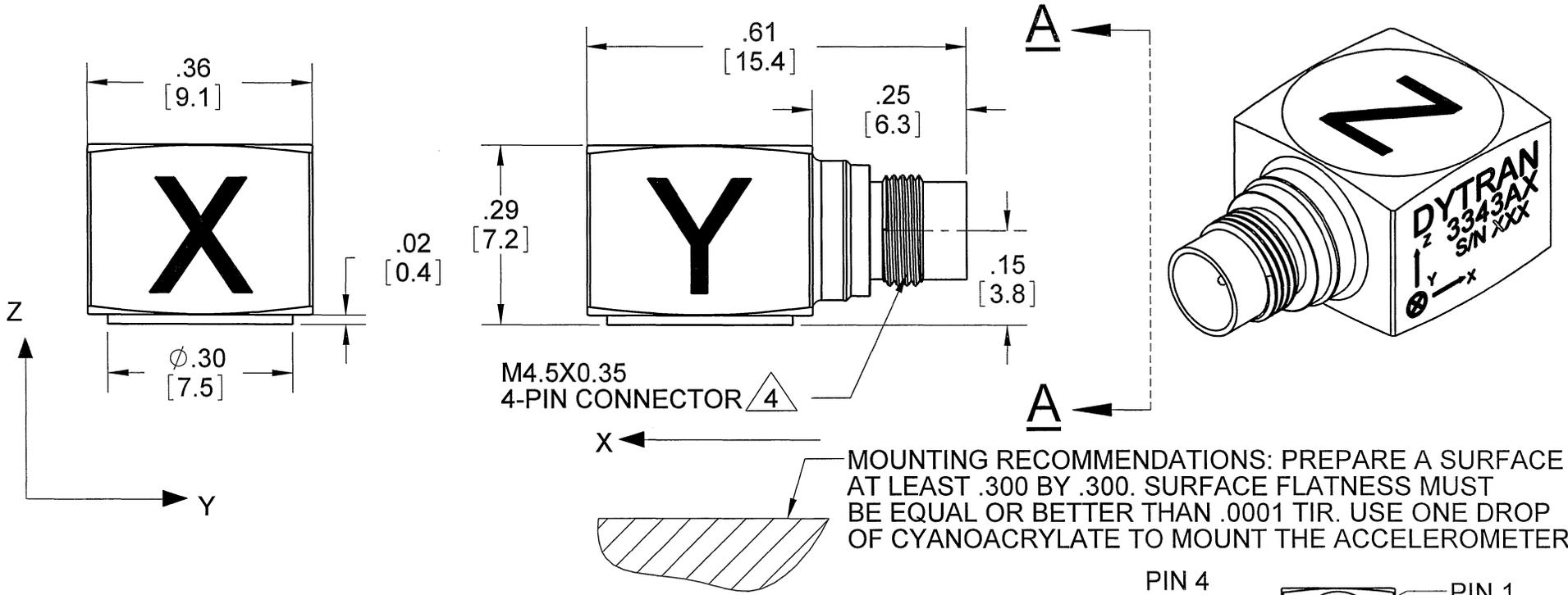
**MOUNTING RECOMMENDATIONS: PREPARE A SURFACE AT LEAST .300 BY .300. SURFACE FLATNESS MUST BE EQUAL OR BETTER THAN .0001 TIR. USE ONE DROP OF CYANOACRYLATE TO MOUNT THE ACCELEROMETER.**
