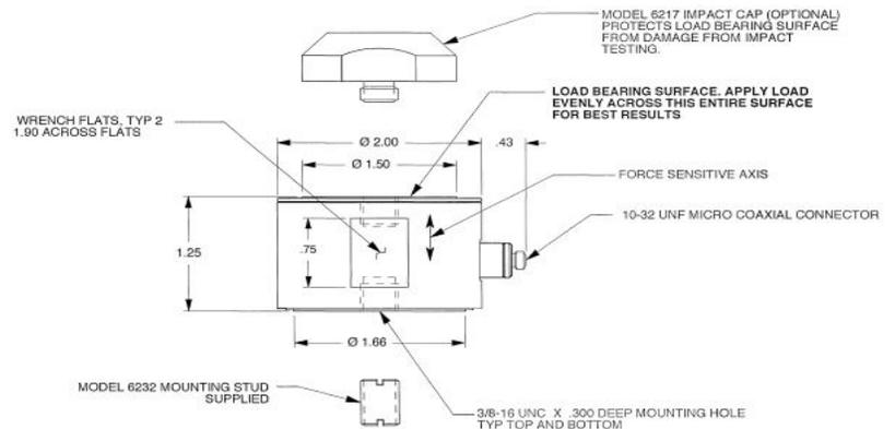
Units on the line drawing are in inches, units in brackets are in millimeters. Refer to 127-1061V for more information.
