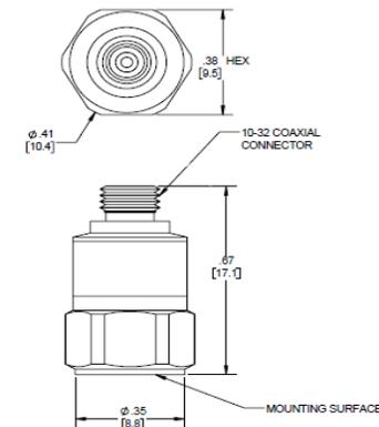
Units on the line drawing are in inches, units in brackets are in millimeters. Refer to 127-3030BG for more information.
