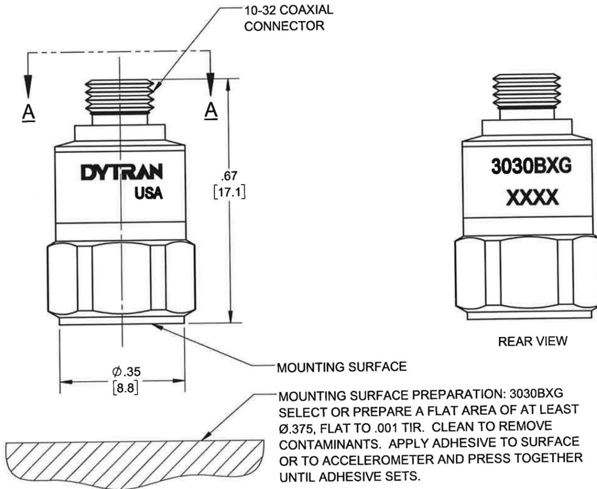
2 ARROW INDICATES SENSE AND DIRECTION OF ACCELERATION FOR POSITIVE - GOING OUTPUT SIGNAL
