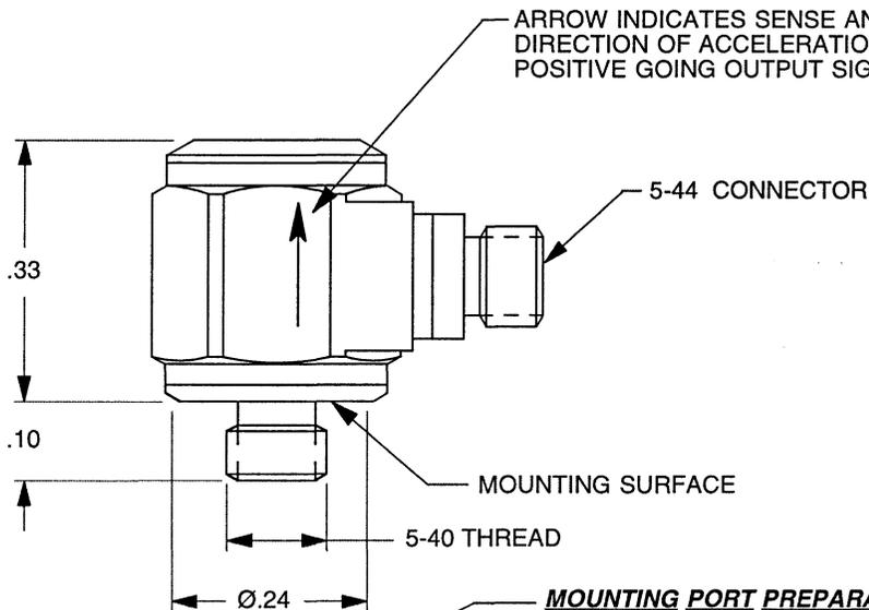
ARROW INDICATES SENSE AND DIRECTION OF ACCELERATION FOR POSITIVE GOING OUTPUT SIGNAL
