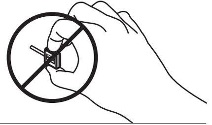
When installing the sensor, connect it to an instrument and monitor the output to prevent possible overload.
