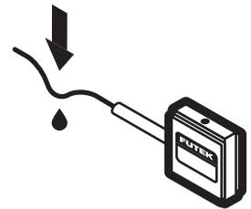
For compression, install the sensor right side up for best results (reference the label). For tension, install the sensor upside down so the load is being applied to the measuring end.
