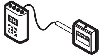
Do not apply excessive torque or create a torque through the sensor when attaching the fixtures.
