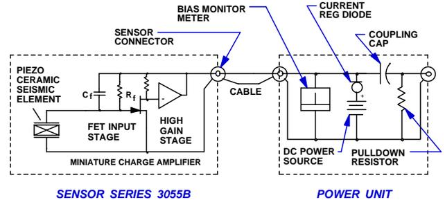
**Figure 1-Electro-mechanical schematic, accelerometer and power unit system.**
