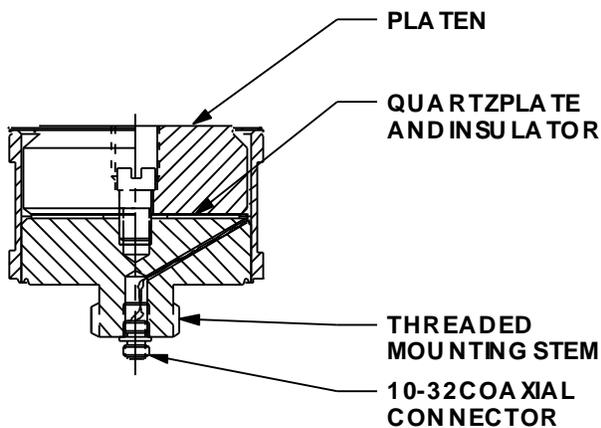
**Figure 1: CROSS SECTION, MODEL 1060C**
