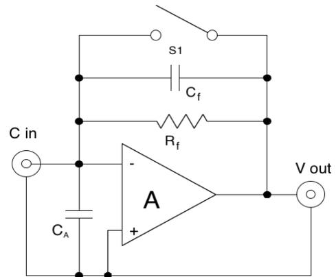
**Figure 2: THE CHARGE AMPLIFIER (SIMPLIFIED SCHEMATIC)**
