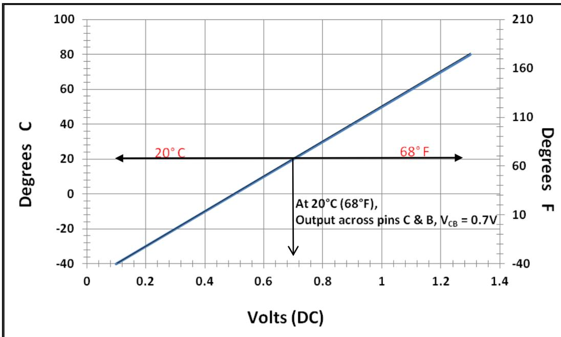
**Figure 2. Graphical representation of the expected Voltage Output at different temperatures (°C or °F)**
