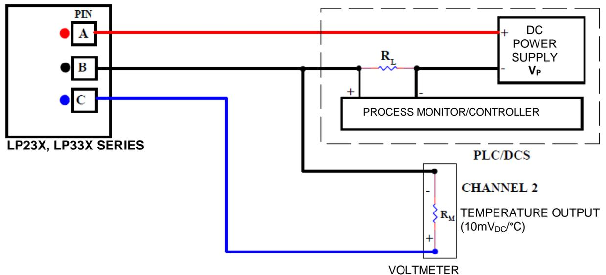
Figure 1. Typical Circuit
